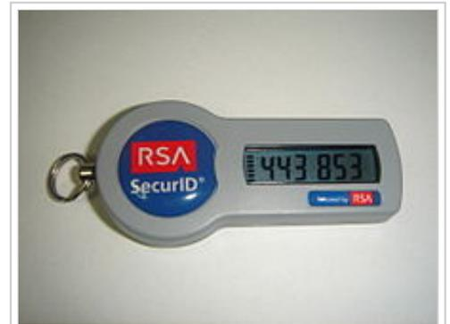
RSA SecurID token, an example of a disconnected token generator.
